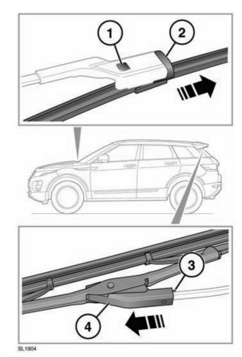
**Rear wiper blade**: Lift the blade clear of the screen.
